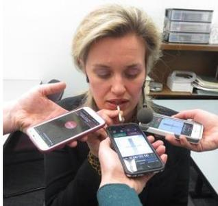
Figure 1. The experimental set-up with the recording devices (iPhone 5 and 6s, Samsung Galaxy S5, head mounted microphone) and the plastic stick that measured 4 cm from the mouth to the microphones.
